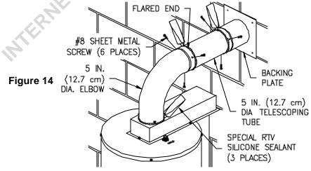
12. Mark the mounting screw hole locations for the backing plate. Rotate the backing plate in order to gain access to the markings. With a 3/16 inch diameter drill bit (not supplied), drill holes for the supplied wall anchors. Install the wall anchors and secure the backing plate to the wall with four (4) #10 x 1 inch screws (supplied) (See Figure 15). Note: Certain construction of walls may require the use of a different type of anchoring means than supplied.
